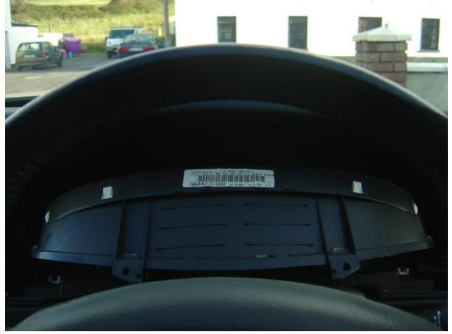
The binnacle is then attached only with its wiring. Just move the clip back and remove>
