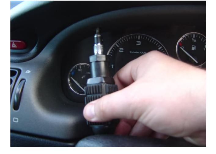
You will be looking then at the binnacle itself. It is attached again with two screws to the top and two either side at the bottom.
